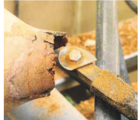
STEP 22. The inside ought to be finished to the best of your ability, and a small teardrop scraper is perfect for this. Speed up the lathe and take light smoothing cuts, being careful not to catch the top edge as you work
